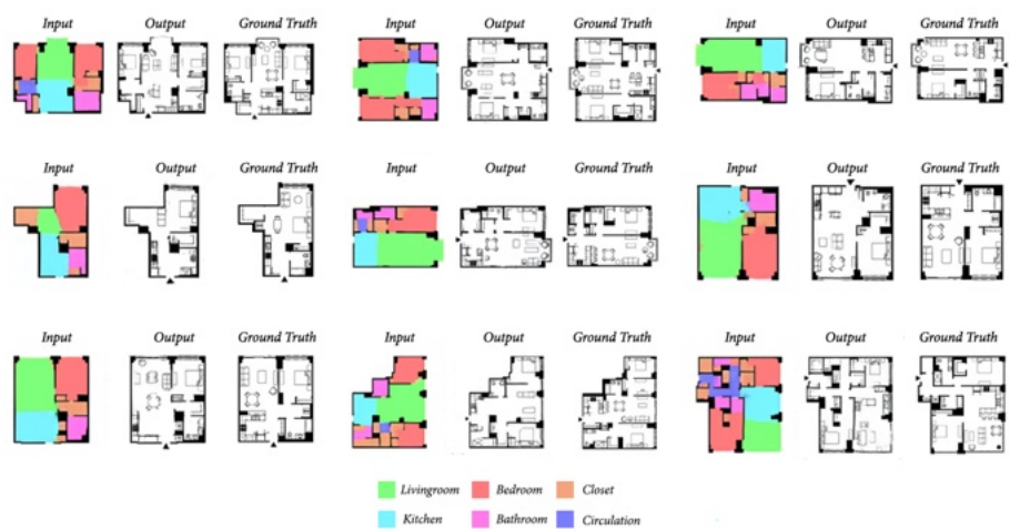
Abbildung 11 Entwurfsprozess Generative Adversarial Networks (GANs). („ArchiGAN: A Generative Stack for Apartment Building Design“ 2019)
