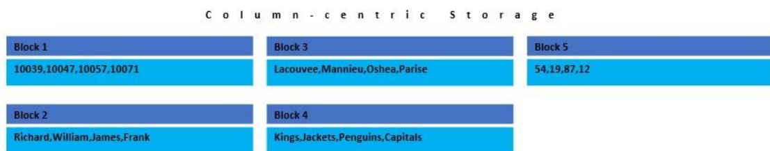
Figure 9: An example of a column-based database elaborated based on the book written by Coronel and Morris (Coronel and Morris 2016, 665)
