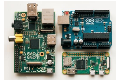
Figure 9: Raspberry Pi 4B, Raspberry Pi Zero and Arduino Uno (Photo by Harrison Broadbent on Unsplash)
